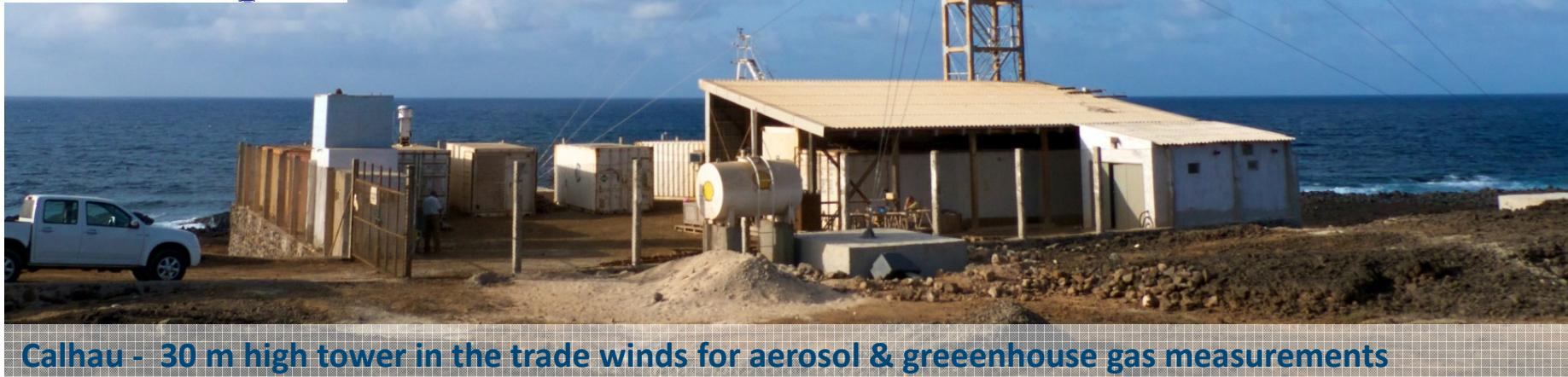
Calhau - 30 m high tower in the trade winds for aerosol & greenhouse gas measurements
