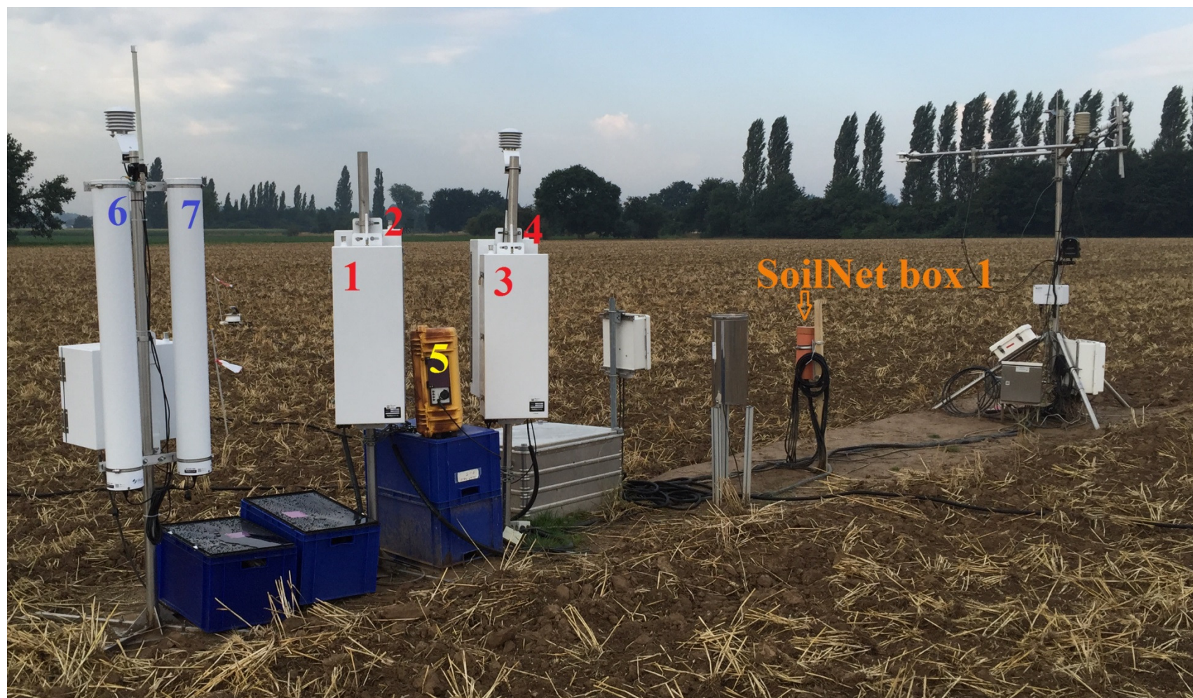
Seven cosmic-ray neutron probes (4 CRS1000, 2 CRS2000/B, 1 cross calibrator)
