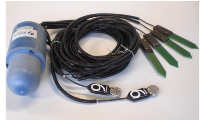
SoilNet sensor unit
