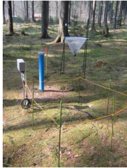
Bodenmessplots (T, SWC, BWS, GW) Biomasse (Dendro, GAI)
